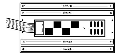
**Bag #40 MASS AIR FLOW SENSOR (MAF):** On a factory installation, this sensor is mounted in the intake air duct between the air cleaner and throttle body. Plug the three gang black connector into the sensor and run the wires back to the panel. Connect the yellow MAF A->1 to #1, black MAF B->30 to #30 and the pink wire MAF C->24 to #24.
