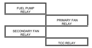
In the cover of the TELORVEK panel are four relays the PCM uses to control fuel pump, primary & secondary cooling fans and the torque converter clutch relay. The PCM can not handle heavy load items and it requires a relay to handle the load and the PCM then controls the relay. The harness has a total of seven relays, four in the cover of the TELORVEK panel and three that are mounted remotely. All relays in the harness require GM part # 14100455.
