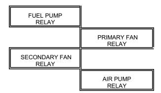
**RELAY CENTER:** In the cover of the TELORVEK panel are four relays the ECM uses to control fuel pump, primary & secondary cooling fans and the air pump. The ECM can not handle heavy load items and it requires a relay to handle the load and the ECM then controls the relay. The harness has a total of six relays, four in the cover of the TELORVEK panel and two that are mounted remotely. All relays in the harness require GM part #14100455, Airtex part #1R1061, Standard Motor Products part #RY116.
