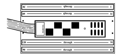
**Bag #20 MASS AIR FLOW SENSOR (MAF):** On a factory installation, this sensor is mounted in the intake air duct between the air cleaner and plenum. Plug the three gang black connector into the sensor and run the wires back to the panel. Connect the yellow MAF A->6 to #6, black MAF B->26 to #26 and the orange wire MAF C->4 to #4.
