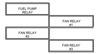
**RELAY CENTER:** In the cover of the TELORVEK panel are four relays the ECM uses to control fuel pump and cooling fan circuits. The ECM can not handle heavy load items and it requires a relay to handle the load and the ECM then controls the relay. The harness has a total of six relays, four in the cover of the TELORVEK panel and two that are mounted remotely. All relays in the harness require Airtex part #1R1061, Standard Motor Products part #RY116 or GM part #14100455.
